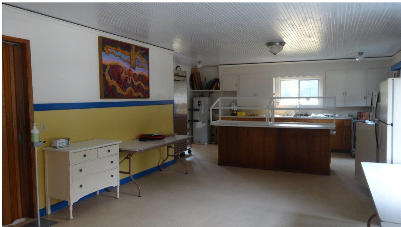
Figure C24. View of kitchen. Note the beadboard ceiling, vertical pressboard walls, and painted upper cabinets that appear to be original.
